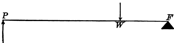
FIG. 41.—A lever of the second order. F , fulcrum; P , power; W , weight. The arrows indicate the direction in which the forces act.
